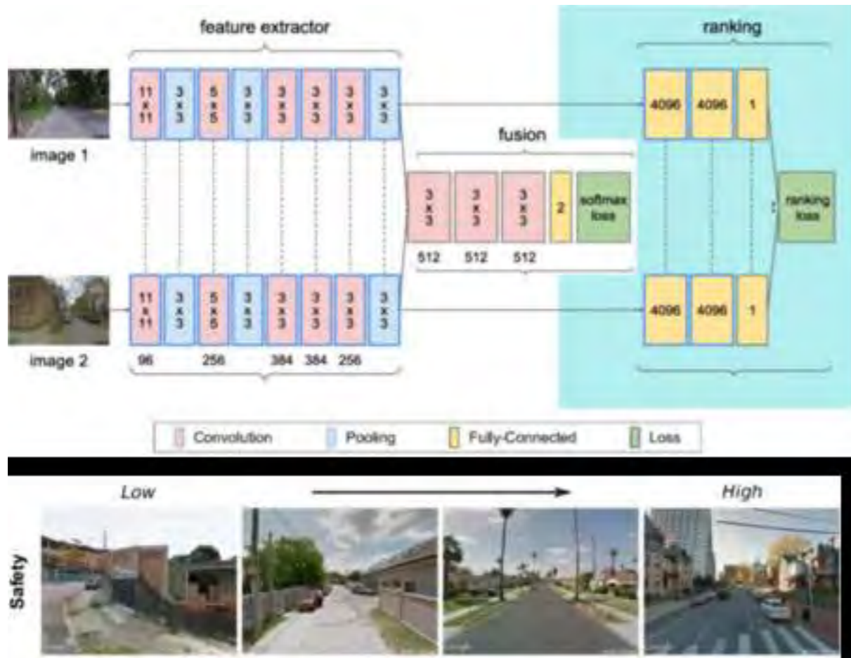
Figure 10. CNN models (Siamese model and Ranking SS-CNN) and Example results generated by the RSS-CNN (Dubey et al., 2016)
